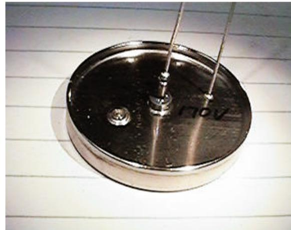
Figure 2. Photograph of the hermetic tantalum Hybrid capacitor.
