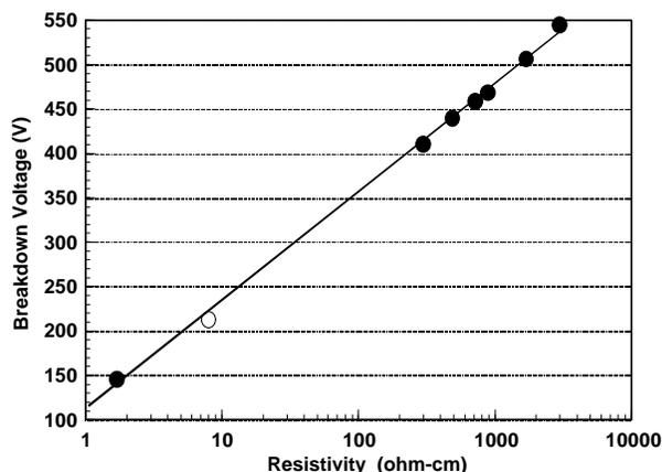
Figure 4. Breakdown voltage vs. Log electrolyte resistivity for  $Ta_2O_5$  dielectric in various aqueous and non-aqueous electrolytes.<sup>3</sup>
