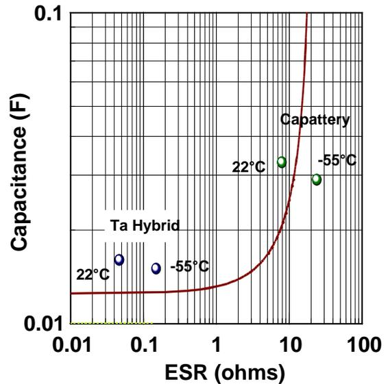
Figure 11. Curve of minimum performance for the missile fuze application. Note that the increase in Capattery ESR at -55°C forces its performance below the curve, whereas a similar percentage change in Hybrid capacitor ESR has little effect on overall performance.
