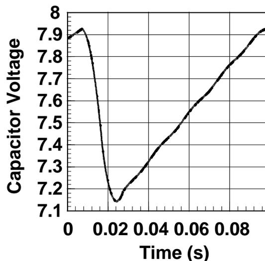
Figure 10. Voltage vs. time for a 45 mF, 8 V tantalum Hybrid capacitor supplying a 3.8 A , 10 ms pulse at a repetition rate of 11 Hz.
