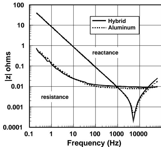
Figure 4. Bode plots for a polypropylene case tantalum Hybrid capacitor and an aluminum electrolytic capacitor, both rated at 54 V, 18 mF.
