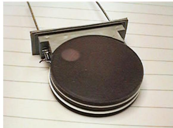
Figure 3. Photograph of a partially dismantled, 3-element polypropylene case tantalum Hybrid capacitor showing stacked arrangement of anode electrodes connected in parallel. The top cathode plate and separator has been removed.
