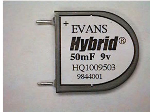
Figure 2. Photograph of the tantalum Hybrid capacitor.
