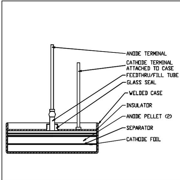
Figure 1. Schematic view showing internal construction of a dual-anode element hermetic tantalum Hybrid capacitor.
