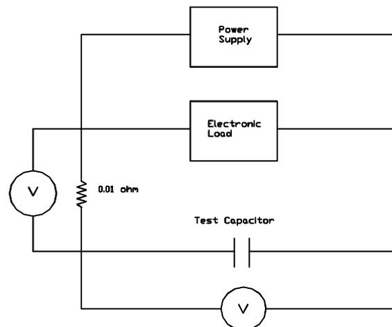
Figure 8. Diagram of the circuit used to measure capacitor performance.
