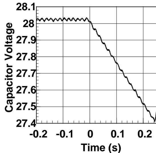
Figure 12. Voltage vs. time for a 17 mF, 28 V tantalum Hybrid capacitor in the missile fuze application. Current pulse is 0.05 A.
