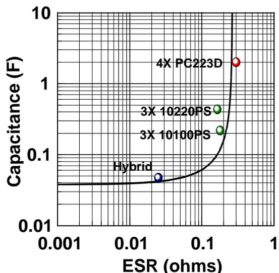
Figure 9. Plot of minimum performance for capacitors in the TDMA-GSM cell phone application. The Hybrid capacitor has a rating of 45 mF, 8 V. The other points plotted are from published data for competing non-aqueous electrochemical capacitors, series-connected (3X or 4X) to provide 8 V operation.
