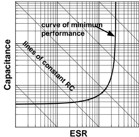
Figure 7. Log-Log Capacitance vs. ESR plot for the ideal RC model. Capacitors which coordinates fall above and to the left of the curve of minimum performance will work in the application.
