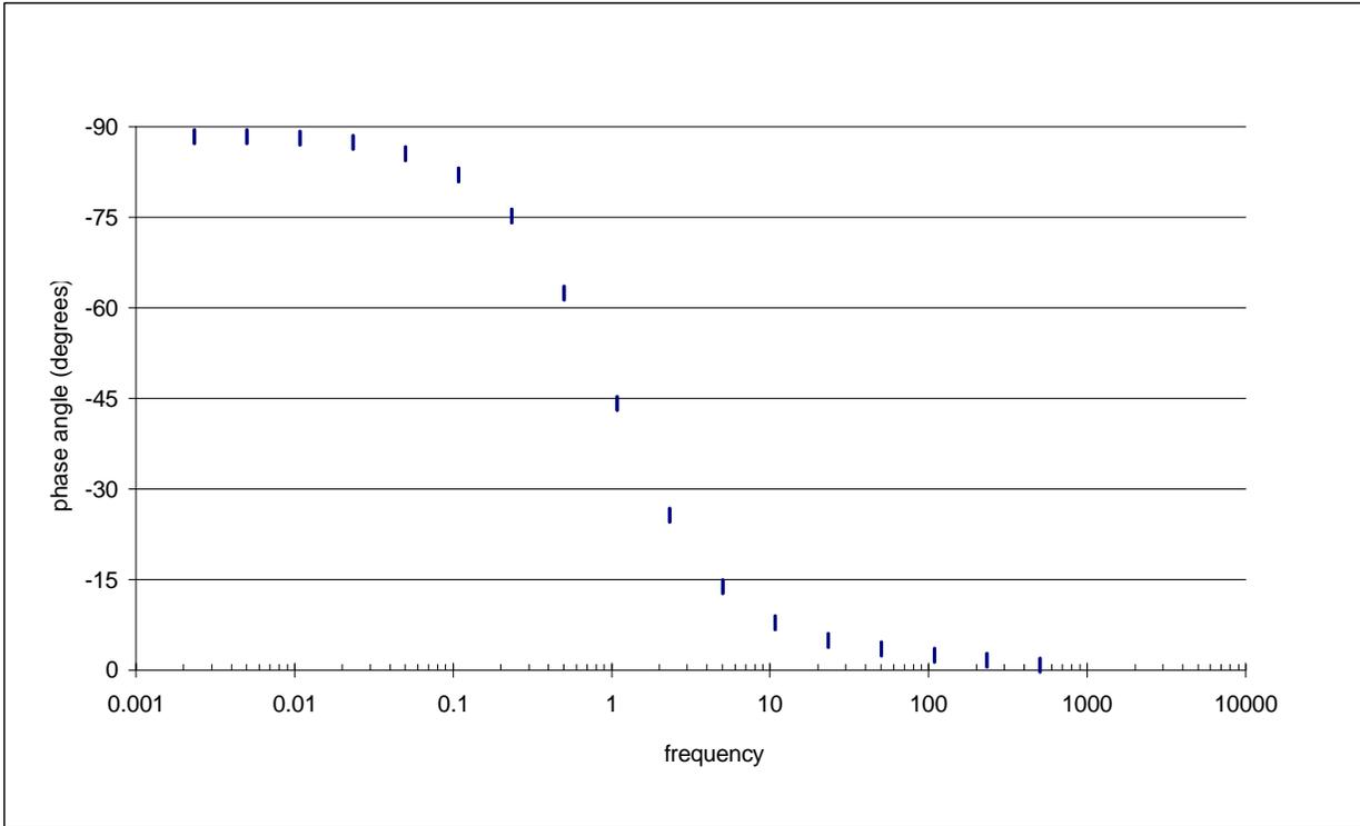
Figure 16. Phase angle vs. frequency for the twelve-cell symmetric particulate amorphous RuO<sub>2</sub> shock-hardened capacitor prototype.
