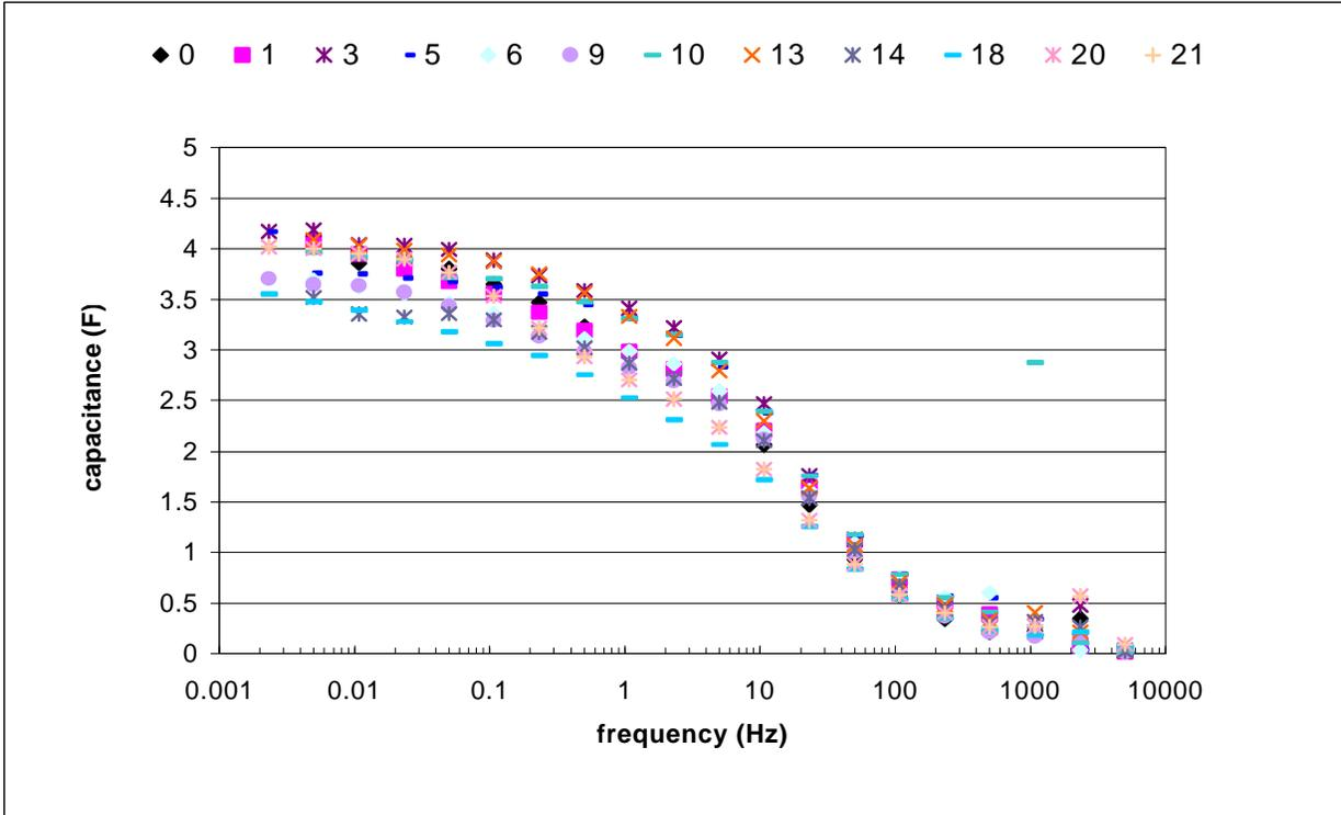
Figure 12. Capacitance vs. frequency for the twelve symmetric particulate amorphous RuO<sub>2</sub> cells used in the shock-hardened capacitor prototype.
