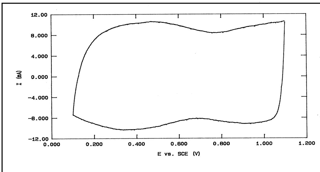
Figure 5. Cyclic voltammogram of amorphous ruthenium oxide electrode in 38 wt.%  $H_2SO_4$  electrolyte at a voltage scan rate of 2 mV/sec. The electrode was made with 6.86 mg of ruthenium dioxide powder and 0.34 mg of Teflon as binder.
