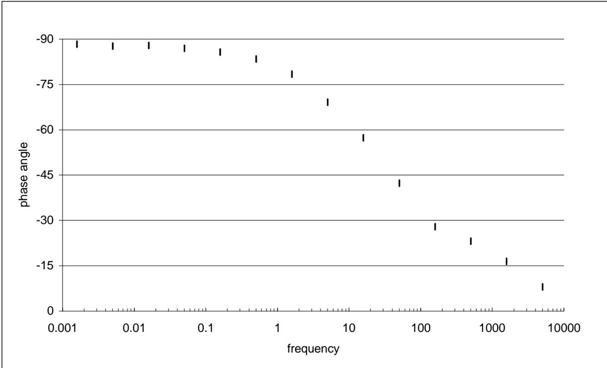
Figure 20. The above figure represents phase angle vs. frequency for the tantalum hybrid capacitor . The phase angle is between  $-85^\circ$  and  $-90^\circ$  from  $\sim 1$  Hz down. This unit has a  $-45^\circ$  phase angle at 65 Hz.
