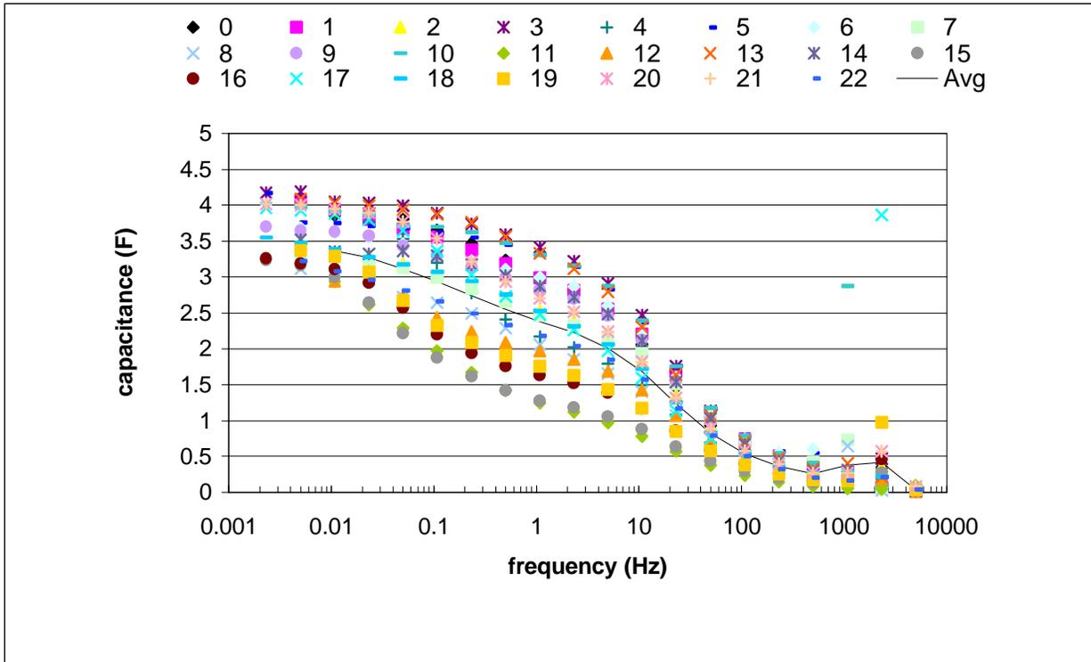
Figure 10. Capacitance vs. frequency for symmetric particulate amorphous RuO<sub>2</sub> cells.
