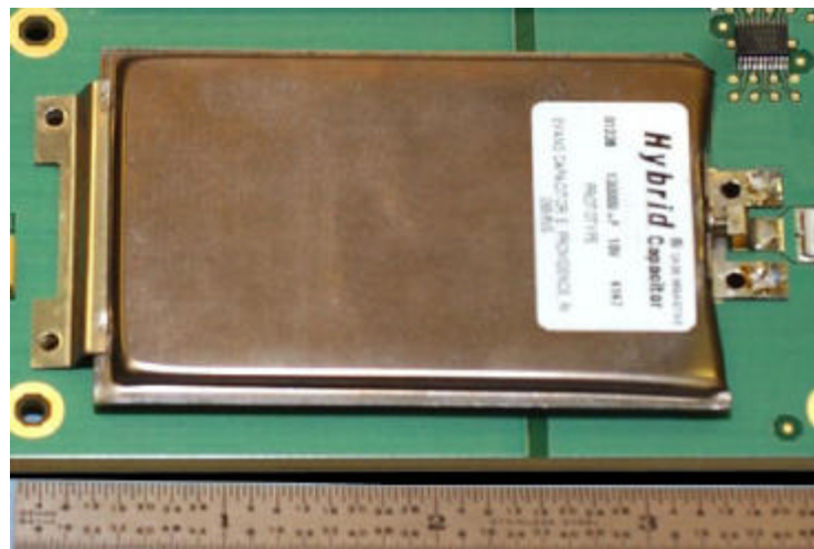
Figure 2. Photograph of the capacitor. The connections are made by soldering directly to the terminals as shown at the right center of the figure. The overall dimensions are 3.07" X 1.98" X 0.21". This device weighs 105g.
