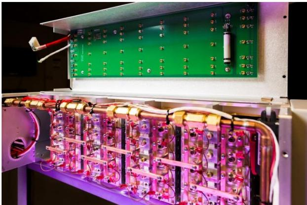
Figure 6 Pulser Crate and Optical Transmitter
