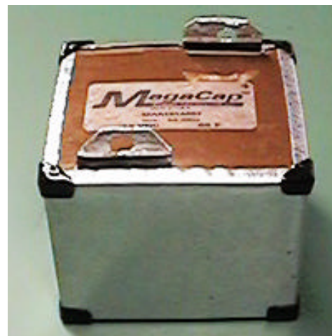
one Fig 1. Photograph of the 15 V, 65 F MegaCap capacitor tested.
