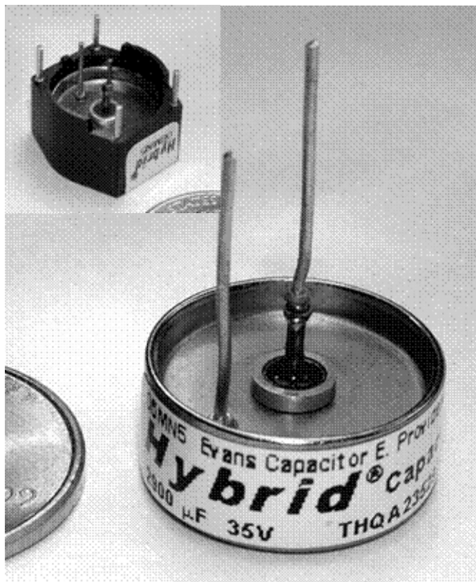
Figure 3. Magnified image of the THQA2. To the left of the capacitor is a US 1¢ piece. The device measures 0.6" diameter X 0.274" high. The weight is 8.7 grams. The inset picture shows the capacitor held in a plastic mount, facilitating PWB assembly by the customer.
