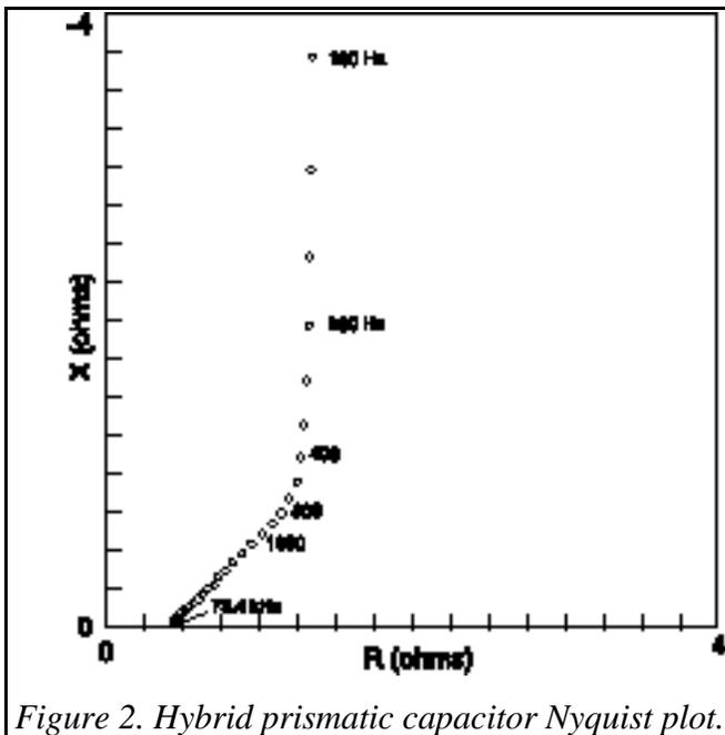
Figure 2. Hybrid prismatic capacitor Nyquist plot.
