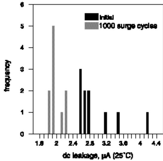
Fig. 10. Surge voltage dc leakage
