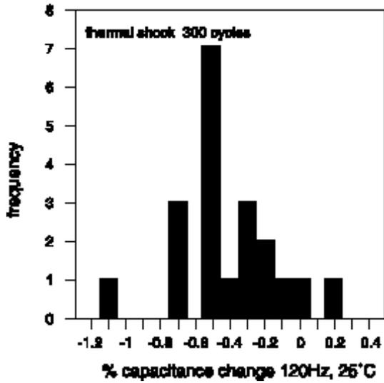
Fig. 11. Thermal shock capacitance change
