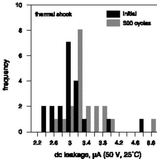
Fig. 13. Thermal shock dc leakage
