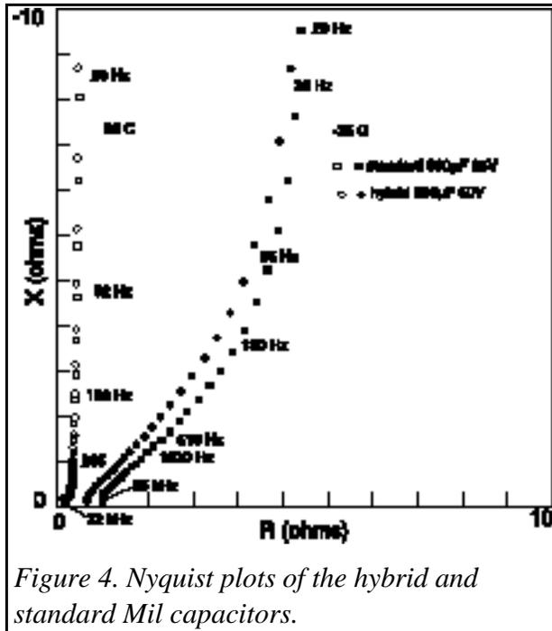
In addition to regular electrical measurements, frequency response analysis was done using a Solartron 1250. The frequency response of the hybrid is compared to that of a 680  $\mu\text{F}$ , 25 V CLR810216, as shown in the Nyquist plots in Figure 4. The frequency response of the hybrid is significantly improved over previous hybrid prototypes and is very comparable to the standard device. This improvement was due mainly to the use of high conductivity sulfuric acid electrolyte.
