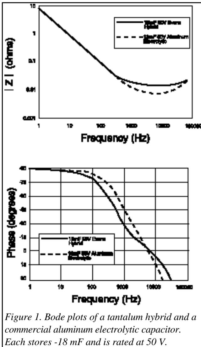
Figure 1. Bode plots of a tantalum hybrid and a commercial aluminum electrolytic capacitor. Each stores -18 mF and is rated at 50 V.
