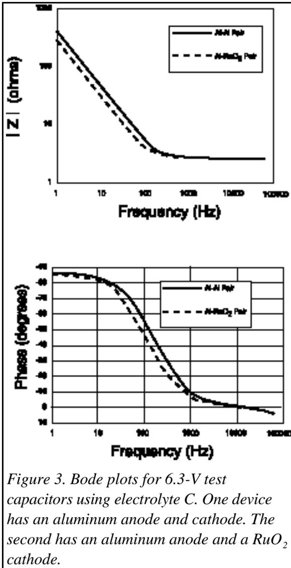
Figure 3. Bode plots for 6.3-V test capacitors using electrolyte C. One device has an aluminum anode and cathode. The second has an aluminum anode and a RuO<sub>2</sub> cathode.
