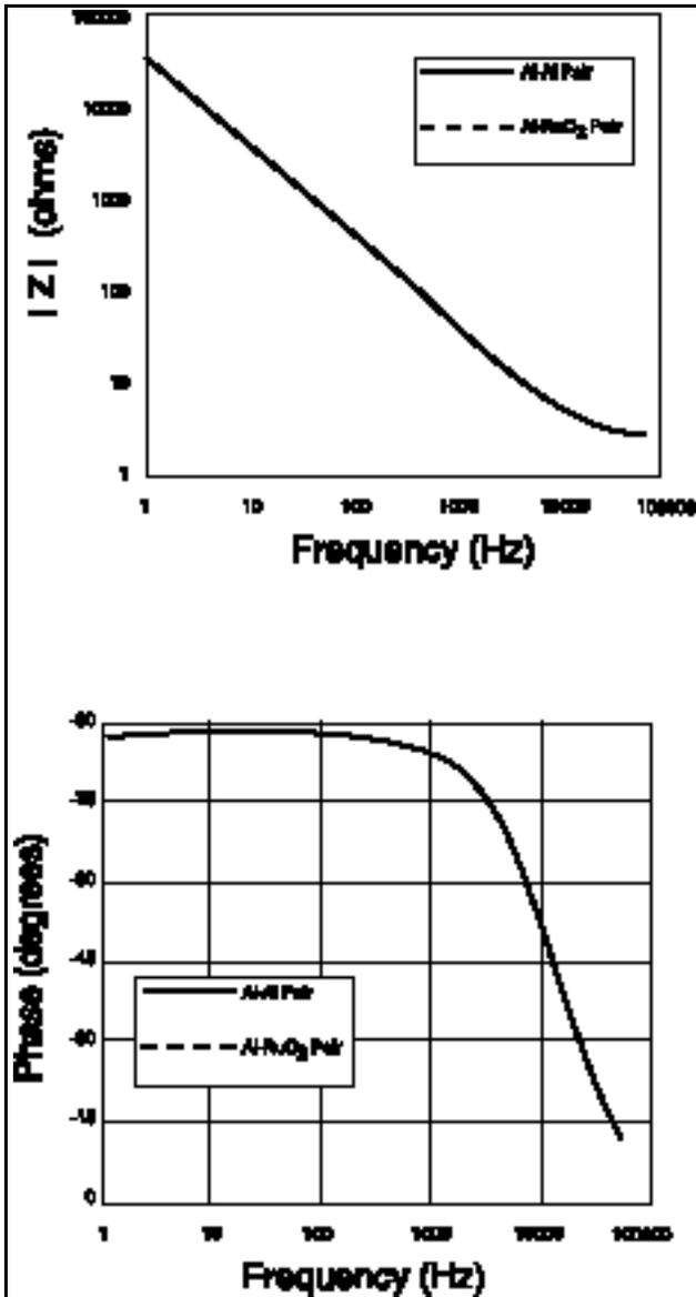
Figure 4. Bode plots for 250-V test capacitors. One device has an aluminum anode and an aluminum cathode. The aluminum hybrid device has an aluminum anode and a RuO<sub>2</sub> cathode. Measurements were made using electrolyte C under ambient conditions.
